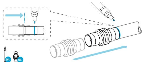
**3** Choose the correct LOKPREP (05) for the tube material and the ambient temperature. Apply LOKPREP (05) all the way round the sealing area of the tube end. Respect the correct curing time of the LOKPREP (05).
