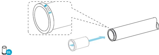
**2** Before applying the LOKPREP (05), push the joint (06) onto the tube until you can feel the inner stop. Mark (04) the correct insertion depth on the tube.
