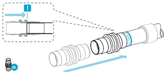
**5** Put the assembly jaws (08) in place behind the LOKRING (07) and the assembly stop of the joint (06). Press the tube connection together. **!** Do not change the insertion depth of the tube and joint (06). Press the tube connection until the LOKRING (07) is flush to the assembly stop of the joint (06). Respect the curing time of the LOKPREP (05) before applying forces to the connection.
