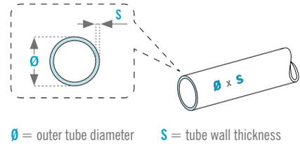
**1** Insert a stabilisation insert (03) suitable for the material, the outer tube diameter  $\emptyset$  and tube wall thickness  $S$ . Stabilisation inserts (03) may not be necessary in case of use with refrigerants with an operating pressure lower than 25 bar (e.g. R134a car A/C systems or refrigerator cabinets).
