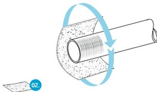
**!** Determine the tube wall thickness  $S$  and the outer tube diameter  $\emptyset$  on the basis of tube coding or using a slide gauge.
