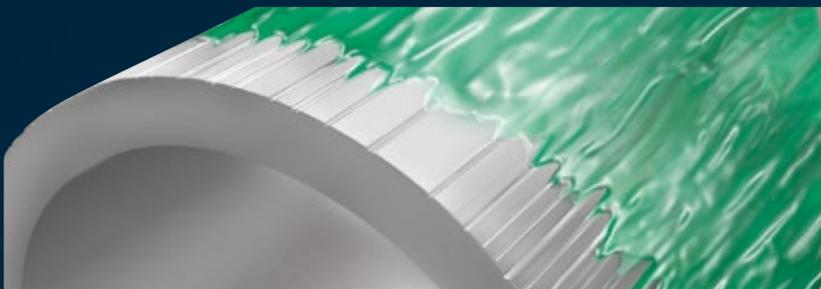
Metal tubes can have longitudinal grooves on the surface from production. These production-related faults can be compensated quite easily by moistening the tube ends to be connected with LOKPREP fluid before assembly. Thanks to its capillary characteristic, it can even flow into microscopic cavities and fill these out completely. LOKPREP is not an adhesive, rather an anaerobic sealant which hardens under oxygen exclusion and in contact with free metal ions.
